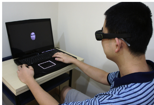
Fig. 2. Image of experimental set-up depicting participant equipped with 3D Vision wireless active shutter glasses. The experiment was conducted in a dark room to minimize reflections of surrounding objects.
